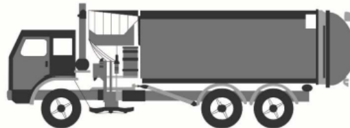
Side-loading waste collection vehicle
